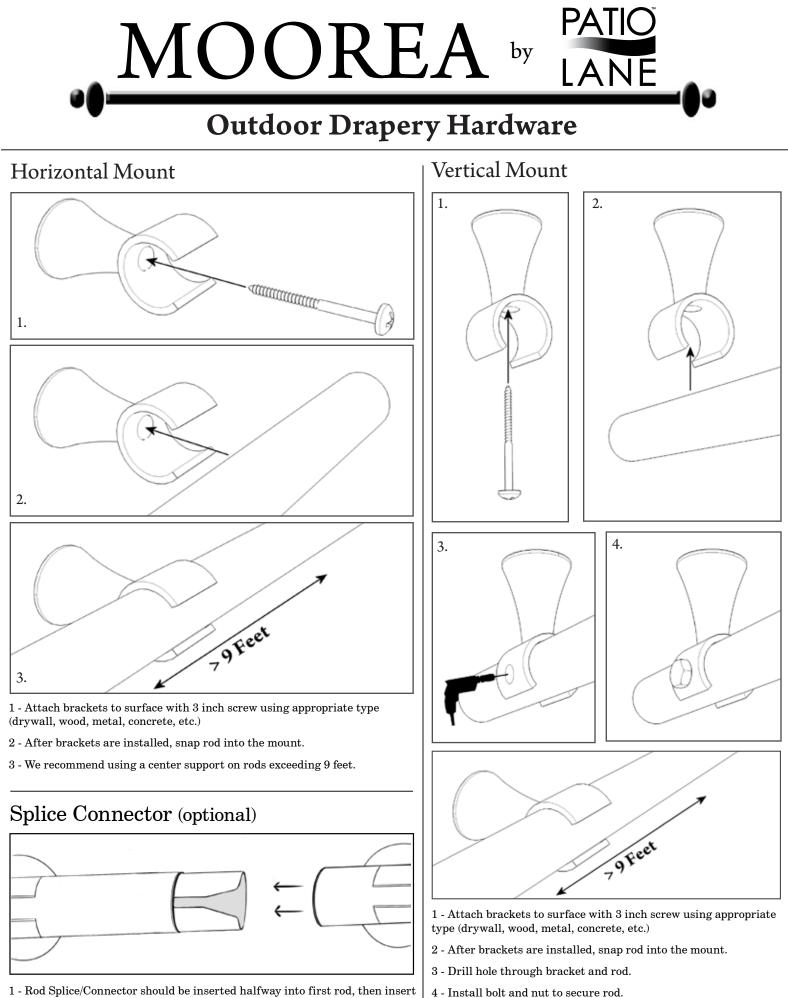
1 - Rod Splice/Connector should be inserted halfway into first rod, then insert remaining into the second rod.
